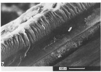
Figure 5 Scanning electron micrographs of fracture surface of partially swollen tapes in dekalin showing the presence of distinct swelling fronts; (a) Hostalen GUR tape immersed at 130°C for 10 s; (b) 006-60 tape immersed at 100°C for 40 s
