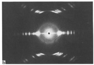
Figure 10 Wide-angle X-ray diffraction; (a) Swollen, dried and unoriented tape. (b) Swollen and drawn (draw ratio=30). (draw direction is vertical)
