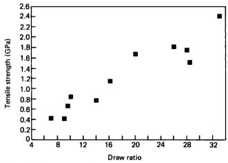
Figure 8 Strength versus draw ratio for Hostalen GUR tapes of initial thickness 0.3 mm immersed in dekalin for 2 min at 120°C
