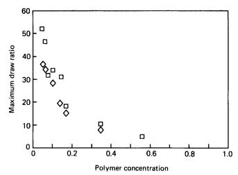
Figure 6 Maximum draw ratio *versus* initial solvent concentration for swell drawn Hostalen GUR tapes; ( $\square$ ) draw temperature = 120°C, ( $\diamondsuit$ ) draw temperature = 90°C
