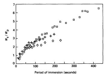
Figure 2 Solvent uptake curves for H060-45P tapes, 0.3 mm thick in xylene; (□) 100°C, (+) 105°C, (⋄) 110°C
