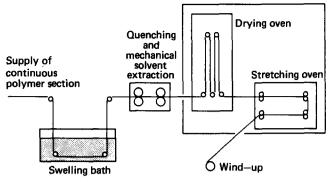
Figure 13 Schematic diagram of a swell drawing process
