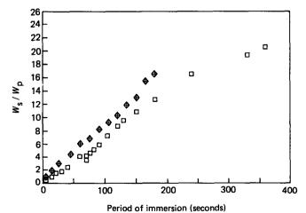
Figure 4 Solvent uptake curves for Hostalen GUR 415 tapes, 0.3 mm thick in dekalin; (□) 120°C, (♠) 130°C
