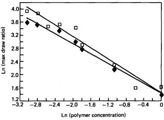
Figure 12 Ln of maximum draw ratio *versus* ln of the initial polymer concentration of swell drawn tapes; ( $\square$ ) draw temperature = 120°C; ( $\spadesuit$ ) draw temperature = 90°C
