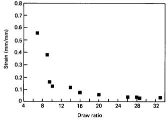
Figure 9 Maximum strain at failure versus draw ratio for Hostalen GUR tapes of initial thickness 0.3 mm immersed in dekalin for 2 min at 120°C
