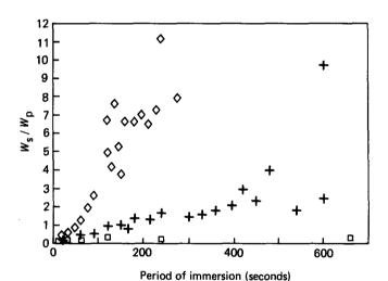
Figure 3 Solvent uptake curves for Hostalen GUR 415 tapes, 0.3 mm thick in xylene; (□) 100°C, (+) 105°C, (⋄) 110°C
