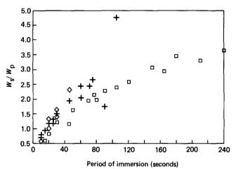
Figure 1 Solvent uptake curves for 006-60 tapes, 0.3 mm thick in xylene; (□) 100°C, (+) 105°C, (⋄) 110°C
