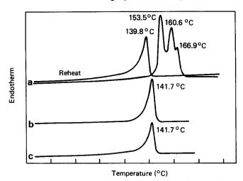
Figure 11 D.s.c. traces, carried out at a heating rate of 10 deg/min on approximately 2 mg samples; (a) Hostalen GUR tape swollen to  $W_{\rm s}/W_{\rm p}=17$  and drawn ( $\lambda=30$ ) with a superimposed trace of the same sample being reheated after cooling. (b) Tape which has been swollen to  $W_{\rm s}/W_{\rm p}=17$  and dried without drawing. (c) Tape as received
