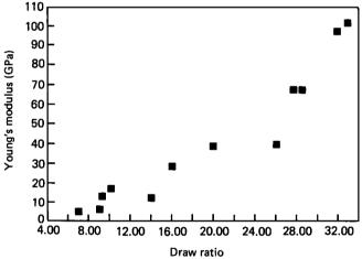
Figure 7 Youngs modulus *versus* draw ratio for Hostalen GUR tapes initial thickness of 0.3 mm immersed in dekalin for 2 min at 120°C
